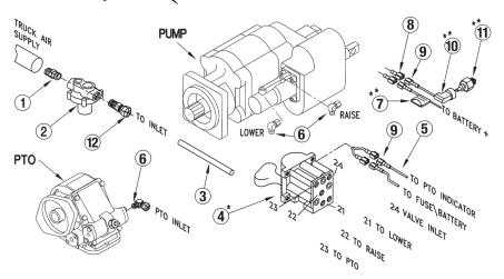
The PTO indicator light must be installed so that it is visible to the operator of the vehicle while seated in the driver's seat. Additional indicator lights may need to be purchased to comply with this requirement.
