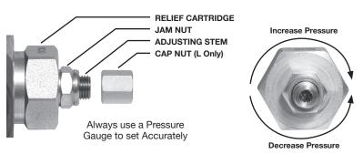
Pump Relief Valve should be set 100 PSI higher than any secondary relief down stream in system.
