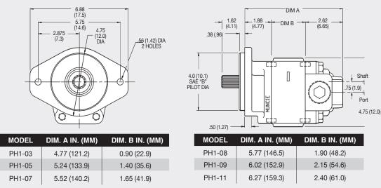
Note: SAE "B" pilot shown. SAE "A" pilot diameter is 3.25 (82.5), .44 diameter holes on 4.19 bolt circle.
