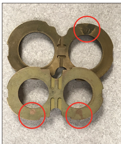
Wear plates from gear pump showing damage from cavitation.
