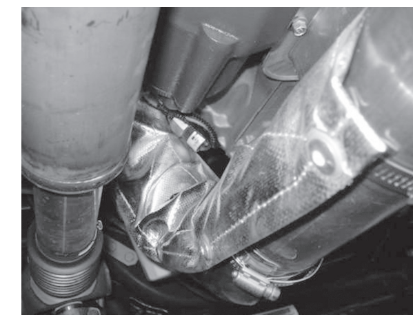
Figure 11. Proper heat shield installation.
