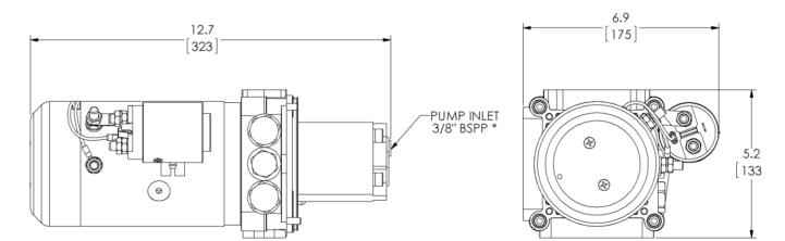
\* P/N BPMJ68P BSPP TO JIC CONVERSION FITTING PROVIDED STANDARD
