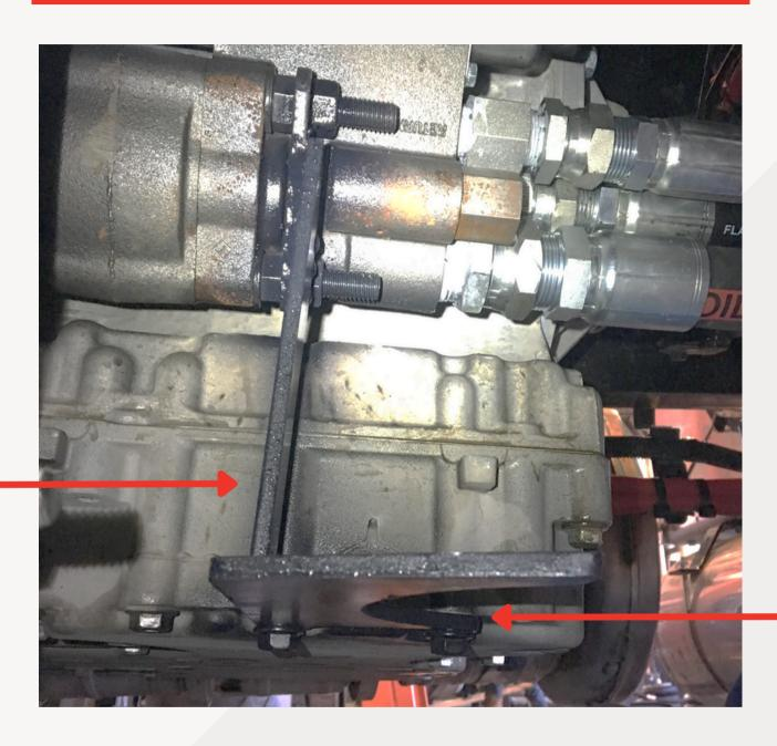
No gussets to prevent flexing at welded corners. Therefore, the bracket will flex as the truck bounces.
