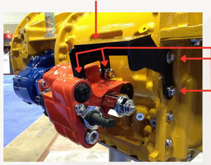
Mounted to two points on both pump and transmission.
