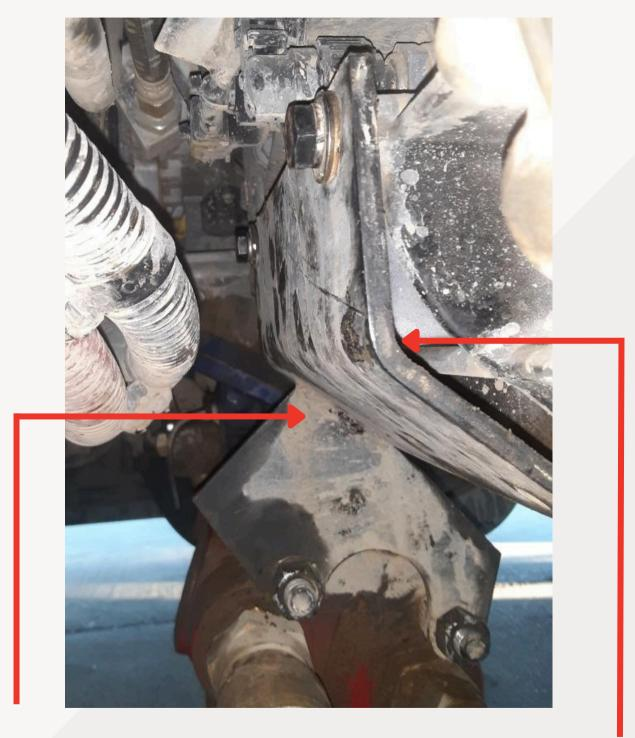
No gussets to prevent flexing at welded corners. Therefore, the bracket will flex as the truck bounces.
