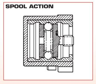
• Specialty Work Sections: Some work sections have special machining characteristics to provide additional features such as reduced pressure drop, load sensing, or load sensing with pressure compensation. Also most work sections are available with machined pilot passages for use with hydraulic remotes or solenoids.
