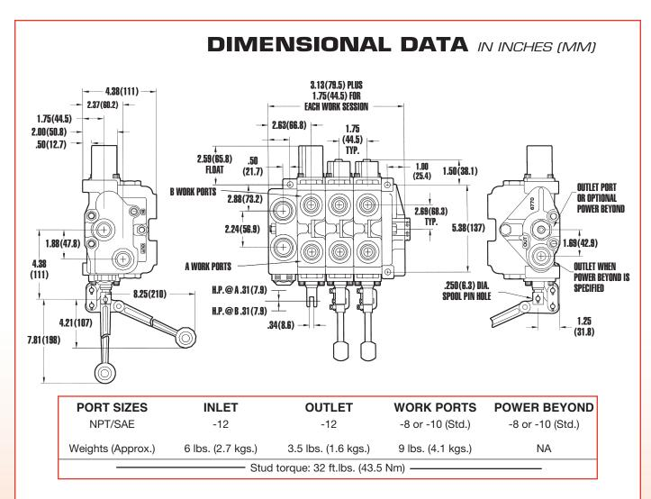
Note: Information shown for standard components. Not all port sizes available in NPT thread. Different assemblies and options could affect weight.
