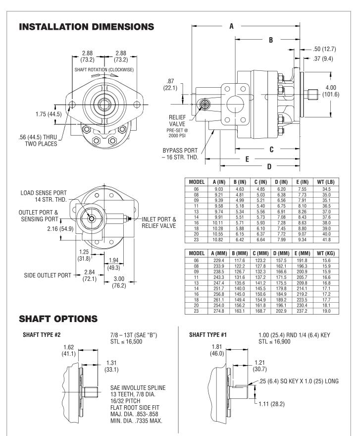
**Shaft Torque Limitations** The pump input shaft can withstand torques up to the designed shaft torque limitation (STL). This figure is based on multiplying the pump cu. in. displacement x the pump pressure (IE:  $D \times P \leq STL$ ).
