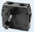
Priority Flow Divider valve provides simultaneous flow for two separate hydraulic circuits from a single pump. The priority flow is adjustable from 0 to 30 GPM (114 LPM). The excess or bypass flow can be used in a second circuit or directed to reservoir.
