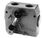
Priority Flow Divider valve provides simultaneous flow for two separate hydraulic circuits from a single pump. The priority flow is adjustable from 0 to 30 GPM (114 LPM). The excess or bypass flow can be used in a second circuit or directed to reservoir. Max. Flow – 30 GPM (114 LPM) Max. Pressure – 3,000 PSI (207 BAR) Ports – 34" N.P.T. or 0.D.T. **RV-30, RV-60** Pilot Operated Relief Valves
