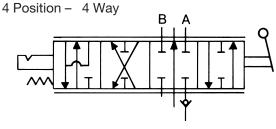
For single or double acting cylinders with 4th position work ports open to tank.
