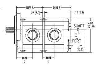
Double Pump Overall Length = A+B First Section Port Centerline = C Second Section Port Centerline = A+D
