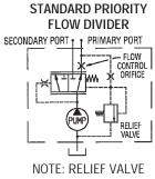
NOTE: RELIEF VALVE BYPASSES FLOW TO THE SECONDARY PORT
