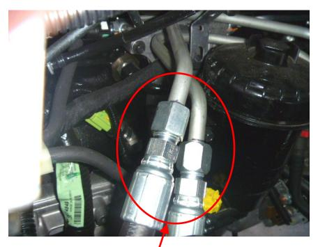
Cut transmission cooler lines and install hoses using the compression fittings making sure to get them tight enough without collapsing tube to prevent leaking.
