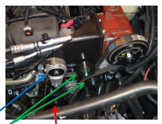
Remove harmonic balancer bolt. Install new drive pulley(1) using bolt(2) and flat washer(3). Torque bolt(2) to 135 ft/lbs. Install set screws(4) into pulley(1) screwing them in finger tight. Cross torque set screws in 20 in/lbs increments until 100 in/lbs is achieved.
