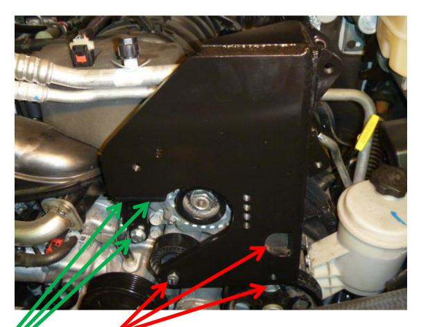
Install main bracket(5) using bolts(7,8,9) and lock washers(10,11). Tighten bolts securely.
