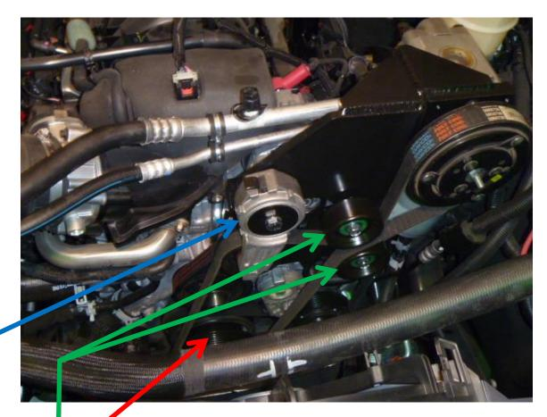
Remove harmonic balancer bolt. Install new drive pulley(1) using bolt(2) and flat washer(3). Before torquing the bolt, rotate the pulley counter clockwise until the drive studs make contact with the spokes in the balancer. Torque bolt(2) to 135 ft/lbs. Install set screws(31), installing finger tight then cross torquing by 20in/lbs increments until 100 in/lbs.
