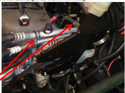
Secure A/C line with the two #10 loom clamps(19) and two 6mm x 16mm flange bolts(20).
