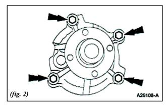
CAUTION! Do not rotate the water pump housing once installed on the engine. Damage to the O-ring can occur, causing the water pump to leak.
