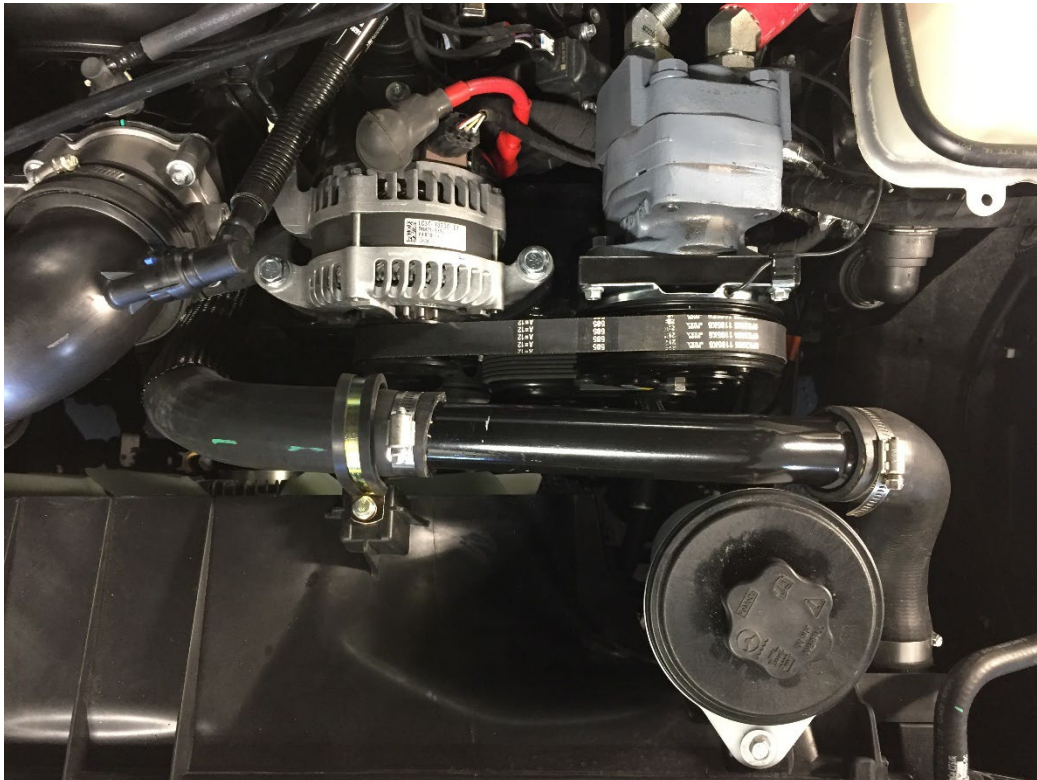
As Shown: Auxiliary Clutch Pump Application
