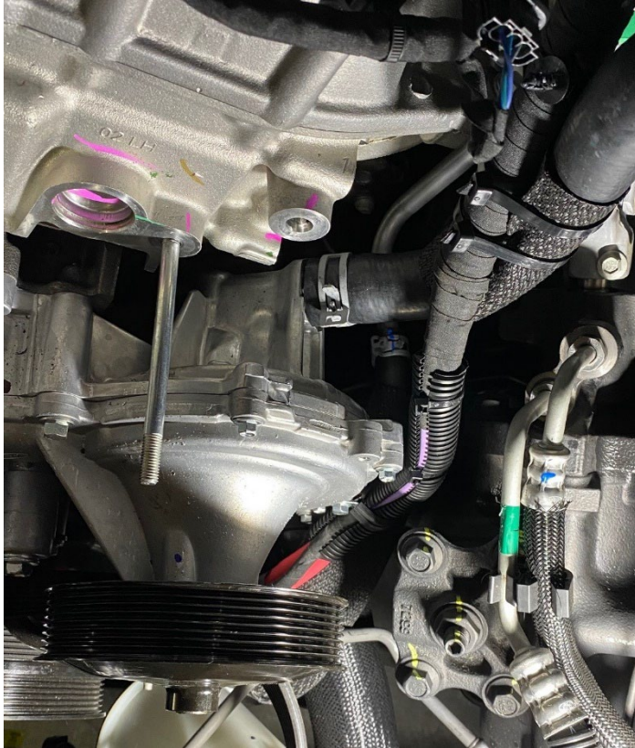
Battery Cable Support Hardware (17-21)
