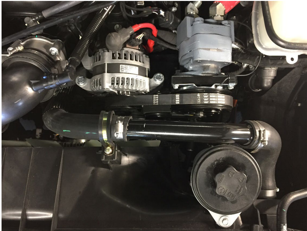
As Shown: Auxiliary Clutch Pump Application
