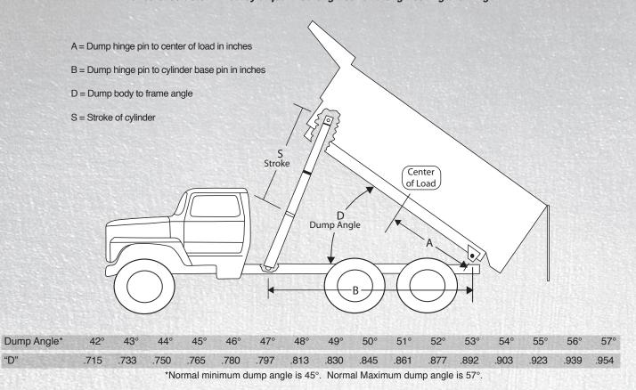
To calculate the appropriate cylinder stroke to achieve a determined dump angle:
