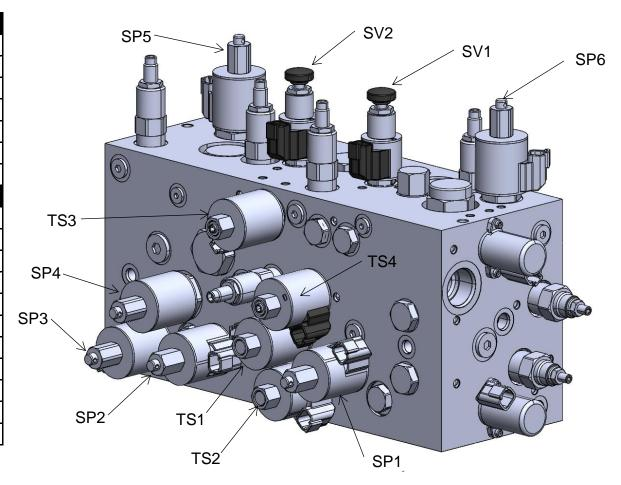
\*Note: To Activate TS3- Main Relief use a 3/16" Allen wrench to turn the Manual Override Screw CW, to fully actuate TS3 turn the screw all the way. After functions have been actuated return screw back to starting position.
