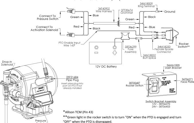
**Note:** Clutchshift PTO's require a connection to the Allison "PTO Enable Input" circuits. Check the vehicle dealer or body builder's information for this location.
