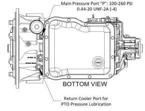
Tee or tap into Return Cooler Port for the PTO pressure lubrication: SAE 8 – 1000 Series (#3 housing) use 43TK5191 tee fitting\* SAE 12 – 1000/2000 Series (#2 housing) use 43TK5157 tee fitting\*
