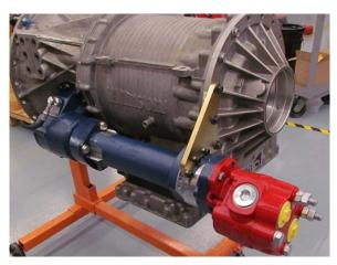
Extended shaft output flanges can be oriented for clearance by removing the capscrews and the flange to the extended shaft housing. Orient the flange and align the bolt holes. Re-install the capscrews and torque to 25 ft.lb.
