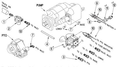
The PTO indicator light must be installed so that it is visible to the operator of the vehicle while seated in the driver's seat. Additional indicator lights may need to be purchased to comply with this requirement.
