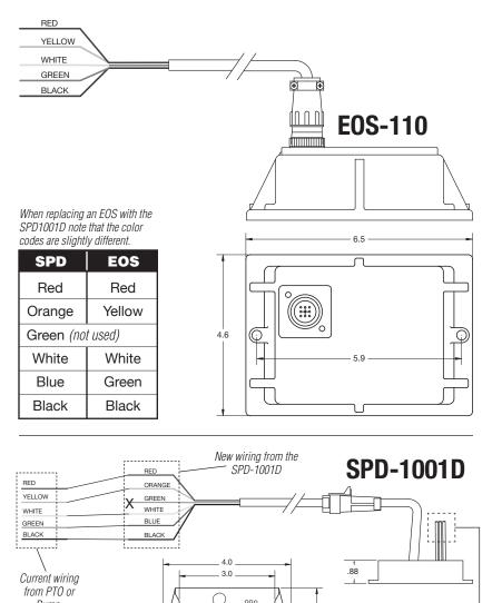
These wires are used for programming the SPD-1001D. They can be cut back after programming is complete.
