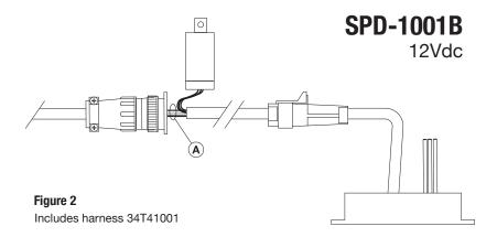
A: For applications needing to control devices using 5A to 10A, use the SPD-1001B, but remove the EOS connector to make your SPD connections.
