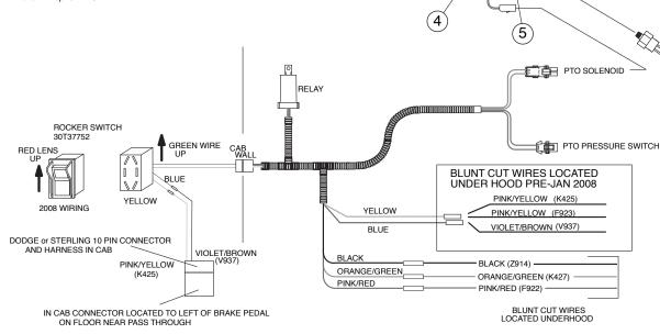
NOTE: The connection made here after Jan. 2008. Only one place is connected — here or under the hood, depending on the date of vehicle manufacture.
