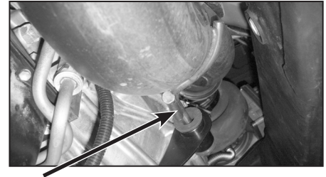
Bar welded to the exhaust pipe and pushed into rubber bushing
