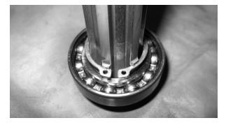
Place the snap ring back onto the shaft with your snap ring tool.
