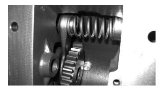
Place the fork (attached to the 25T gear) and the spring down into the PTO housing so the fork's yoke end is towards the shaft as shown.
