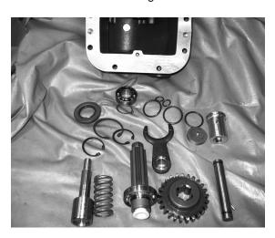
14. This concludes the disassembly of your 8405 Series PTO. All the parts should be present as seen in this photo.
