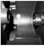
2. Place bearing into the covered end (side opposite of the shaft opening) of the PTO by going through the open shaft end. Use an 82-series bearing driver (or something equivalent) to properly seat the bearing into the PTO housing.
