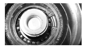
Once the shaft/bearing is properly seating into the other bearing/PTO housing, place the snap ring into the proper groove to secure the assembly.
