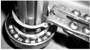
Next, remove the snap ring with your snap ring tool located on the shaft as shown.
