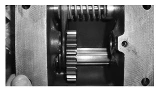
Proceed to remove the input gear, bearings, spacers and the shims. Your PTO housing should look like the picture shown above.
