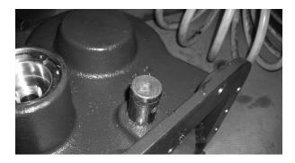
Knock out the idler shaft as shown above. The idler shaft will only be knocked far enough to remove the o-ring as described in the next step.
