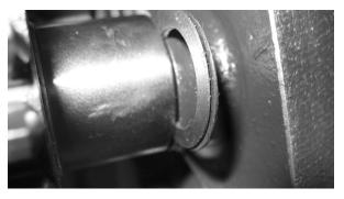
13. Once the idler shaft is lined up from the previous step, begin to properly set in your shims to the required play in the gear as noted above.
