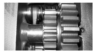
12. Place the spacer next to the gear and continue to slide the idler shaft through the opening (a hammer may be required to continue the idler shaft through the opening). Once the spacer is in place, line up the idler shaft with the end of the spacer to insert the remaining shims.
