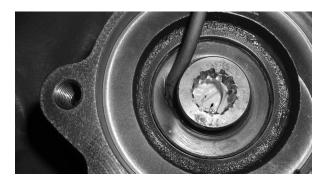
Use a cotter pin extractor (or screwdriver) to remove the seal.
