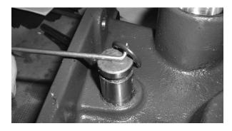
3. Remove the o-ring from the idler shaft and begin to drive the idler shaft opposite of the initial stage.
