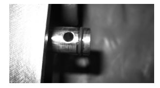
11. Place the remaining o-ring onto the groove located next to the roll pin opening on the idler shaft.
