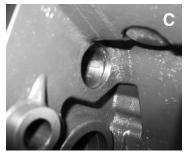
Begin by placing the o-rings back on the parts and the o-ring back into the housing where the piston assembly is located as shown in steps A-C above. One (1) o-ring will go on each of the spring/piston end covers (the o-rings for the idler shaft will be put on later in the assembly).
