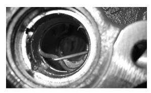
13. Once the rest of the parts have been removed from the spring/piston assembly, the o-ring located in the PTO housing can be removed.
