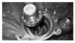
7. Place the bearing onto the shaft and insert the shaft/bearing assembly into the gear, noting the grooves in the shaft going directly into the gear. Apply grease to the internal splines of the output shaft. Use an anti-seize grease or a high temperature, high pressure lithium based grease.
