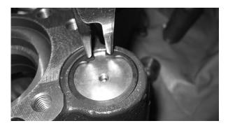
Place the remaining cover for the spring/piston assembly back on where the air activation is located. Just like in step 3, you will have to push the cover down into the PTO housing until you reach the snap ring groove. Once the groove is reached, release the snap ring from the snap ring tool to hold the cover/assembly into place.
