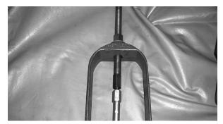
be pulled out. Continue to pull the shaft out until the rear bearing has been popped off of the shaft. These are shown in steps A-D below.
