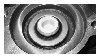
Next, insert the shaft seal over the shaft. Using an 82-series bearing driver (or something equivalent), seat the shaft seal down into the groove of the PTO housing.
