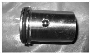
12. The cover on each side can also be removed by threading a screw or bolt into the threaded hole and pulling up until the cover is removed. Removing the rest of the spring/piston assembly can follow once the covers have been removed.
