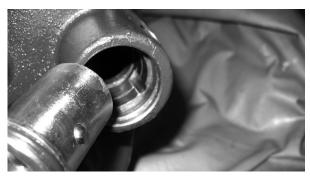
Insert the cover (with the detent ball) into the grooved side opposite of the shaft. Push the cover down into the housing until you are past the snap ring groove and place the snap ring over the cover to keep it into place.
