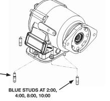
**4.** Remove the inspection cover from the PTO, as shown.
