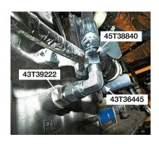
15. "G" Shift option ONLY. Install the 30T60223 pressure switch into the rear cover as shown. Connect the activation pressure port to the fitting installed in the activation port.
