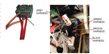
The VSIM comes with 3 harnesses: Green, Brown, and Black. The 16 pin brown harness has an Orange/Brown wire located in Pin #8. This wire is to be connected to the Violet/Yellow wire from the gray connector.
