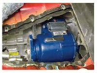
**6.** Check the backlash between the transmission gear and the PTO input gear. The backlash should be between .006 and .012". If not, remove nuts and remove or add gaskets until the proper backlash is achieved.
