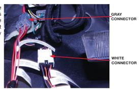
From the Ram Truck wire and harness kit use the 6 terminal gray connector with wires already located in the cavities. Pin# 5 has a Violet/Yellow wire which is to be connected to the Ram Truck VSIM control.
