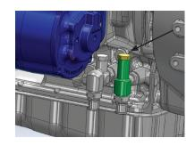
**11.** Install a straight adapter 43T39222 into this port.
