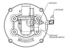
**16.** "G" Shift option ONLY. Connect the lubrication line into the orifice elbow installed on the side of the PTO.
