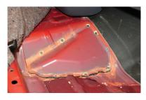
2. Remove this access panel to reveal the right side PTO opening. If you are installing a large pump, then insert it first into the hole and rest it on the exhaust until the PTO is installed. Remove the cover plate from the transmission taking care to avoid possible hot oil coming from the plate and opening. Clean the pad of any debris or sealing material.
