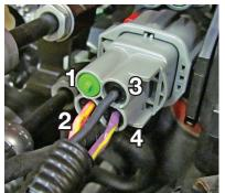
Strip the insulation on these leads ½" for connection to the butt splice.
