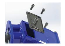
**5.** Place the PTO gaskets over the studs. Place the PTO onto the studs and the PTO pad. Mount nuts onto the red studs as shown in Step 3 (install at 6 and 12 o'clock positions). Torque to 18 ft.lbs.
