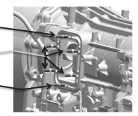
Using the gaskets provided with the PTO, place the gasket over the studs and onto the PTO mounting pad. Torque nuts to 40 ft.lb.
