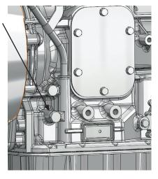
14. Install a straight adapter 43T39222 into the activation port and install a 90 degree elbow 43T36445 into this port. Connect the 36" hydraulic line (45T38840) to the elbow.
