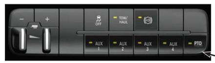
The Ram Truck provided switch allows for PTO operation with throttle advance options. The throttle advance is programmed through the Electronic Vehicle Information Center (EVIC) located in the center display. The 2013 & later vehicle is equipped with an electronic control system called the VSIM. The VSIM can be programmed for a single set speed.
