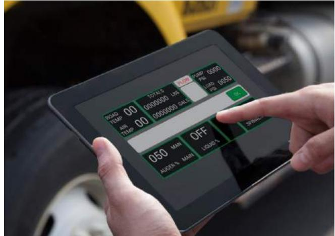
3. **Adjusting Settings** - To adjust spreader speeds or perform a spreader calibration, the spreader control must also be in the configuration menu.
