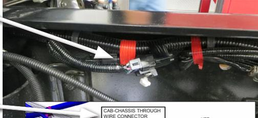
5. Using the Frame half of the harness with the loom, locate the Hino connector along the right side frame rail behind the cab. Remove the blank plug and connect the Muncie Harness.
