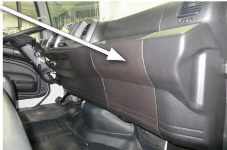
2. Remove the capscrews holding the dash board panel show. Then remove this panel.
