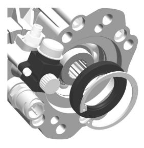
Lubricate the O-Ring on the GB1\* gearbox with transmission oil and mount the gearbox to the PTO using the two mounting capscrews and lock washers provided.
