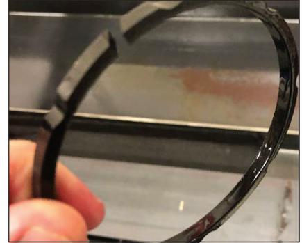
13. Repeat steps 9–12 until all stages have been removed from the cylinder. Always work from the smallest diameter out to the largest diameter stage during disassembly.
