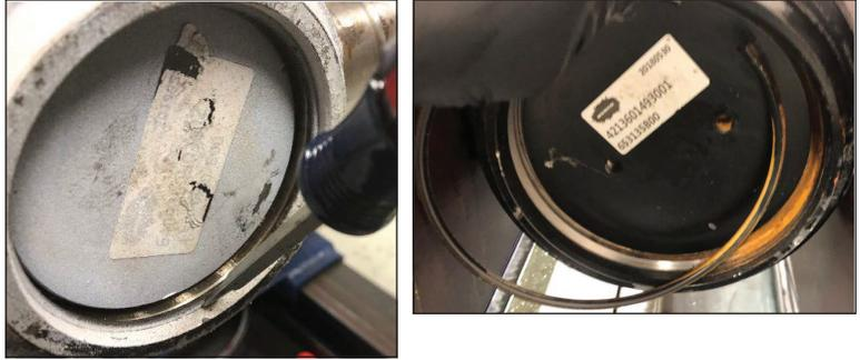
8. Now, remove the base plate using a plate extraction tool, or with a press, push the stages back into the cylinder and press the bottom plate out of the cylinder.
