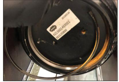
8. Now, remove the base plate using a plate extraction tool, or with a press, push the stages back into the cylinder and press the bottom plate out of the cylinder.
