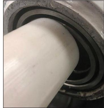
26. Reinstall the base plate by driving it in using the stiff, elastic rod and a hammer. Be sure you have replaced the base plate seal before installing the plate.
