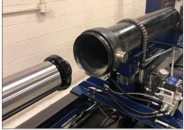
29. Secure the outer cover to the smallest stage by adding the washer and 60mm nut. Use a 60mm impact socket and impact wrench to secure the nut.
