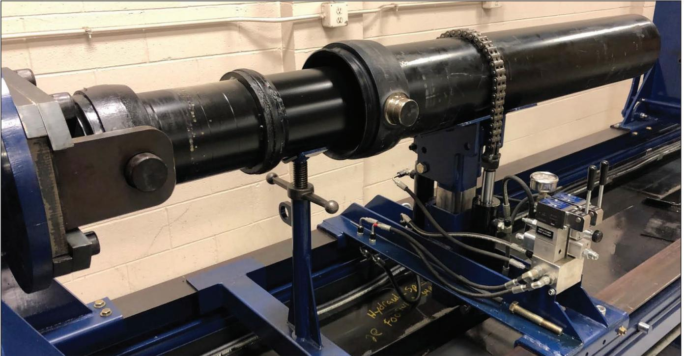
2. Remove the 60mm nut using a wrench or an impact wrench with a 60mm socket.
