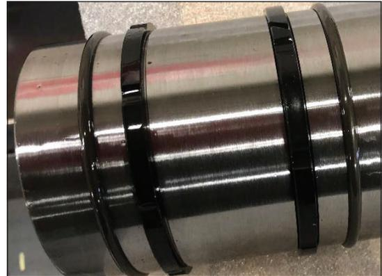
22. Install the next stage into the cylinder. This will require using the stiff, elastic rod and a hammer. Be careful not to damage the stages as you install them into the cylinder. NOTE: You may need to center the stage as you install it, otherwise the stop on the bottom of the stage may catch and prevent the stage from sliding into the cylinder.
