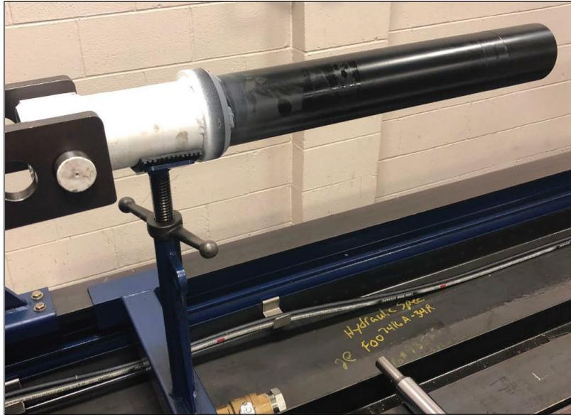
4. Secure the cylinder so that it is possible to begin removal of the stages.
