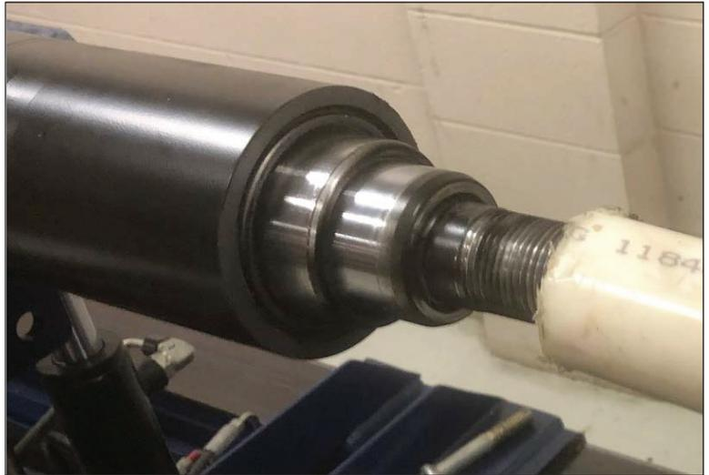
11. Remove the wiper, the guide ring(s), and the high pressure seal from the top end of the stage in the cylinder.
