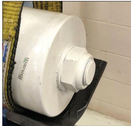
30. If you have the capability to test the cylinder, do so now. Fully cycle the cylinder several times checking for leaks. If a test stand is not available, install into a truck and cycle the cylinder several times. Because the cylinder is self-bleeding, it may take 8–10 cycles before all of the air has bled out.
