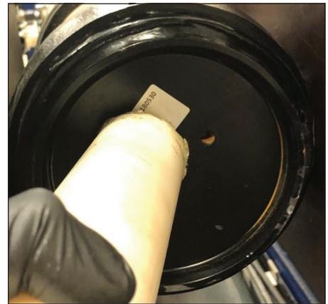
27. Secure the plate by installing the base plate snap ring.
