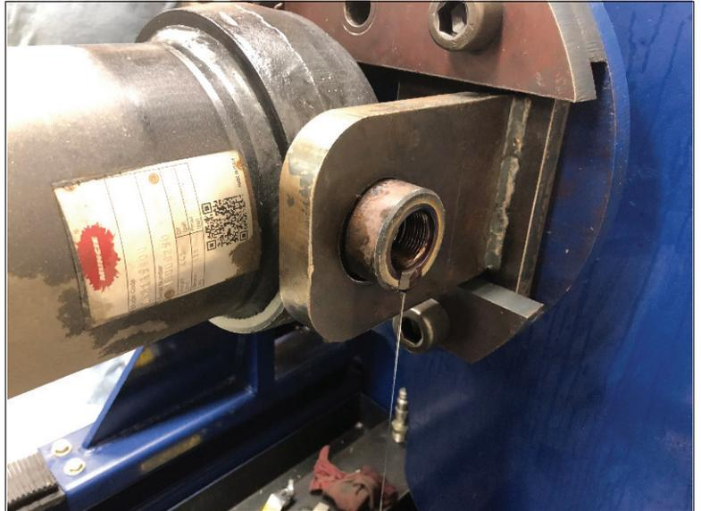
6. At the base of the cylinder, use a stiff elastic rod and a hammer, or make use of a press, to push the bottom plate into the cylinder 0.5–1" to access the snap ring.
