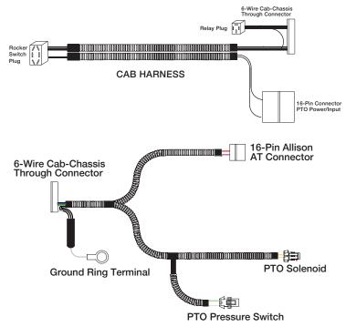
Locate the wiring harnesses provided in this kit. The harness can be separated into two sections. The section without the loom is for inside the cab. Pull the fuse access panel from the dash board.
