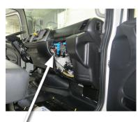
Remove the capscrews holding the dash board panel show. Then remove this panel.
