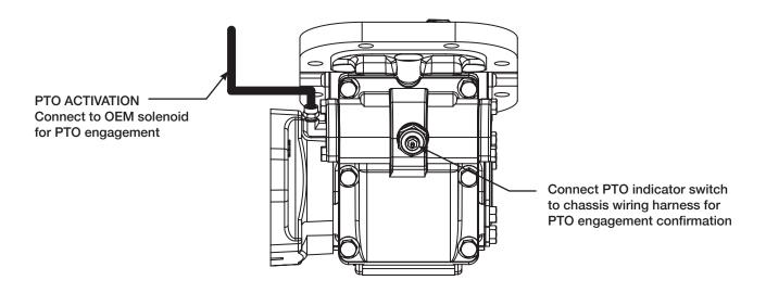
82 Series PTO "P" or "T" Shift Option—REQUIRES VEHICLE ORDERED WITH PTO CONTROL OPTIONS that includes two solenoid operated air valves for DA air cylinder (Note: If the is vehicle ordered with a single solenoid, see page 4 of this document for instructions.)
