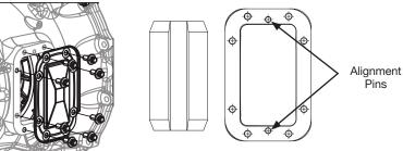
5. Install supplied gasket over alignment pins. A thin coating of approved transmission fluid on gasket is recommended to help hold gasket to opening. Mount PTO with provided cap screws, studs, and nuts. Check for proper PTO fit on transmission prior to tightening down fasteners. PTO mounting surface must be flush against transmission prior to tightening mounting fasteners! Failure to do so may result in damage to PTO
