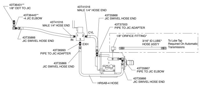
\*SUPPLIED WITH PTO SPECIAL FEATURE OPTION "P" PRESSURE LUBE \*\*ORDERED SEPARATELY FOR ALLISON TRANSMISSION AS SHOWN ON APPLICATION PAGE ALLI-9
