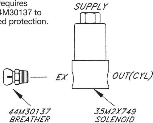
Note: This supplement to be used in conjunction with the original installation instructions. The new solenoid valve being used along with the addition of a breather in the exhaust port(s) is for added protection against contamination.
