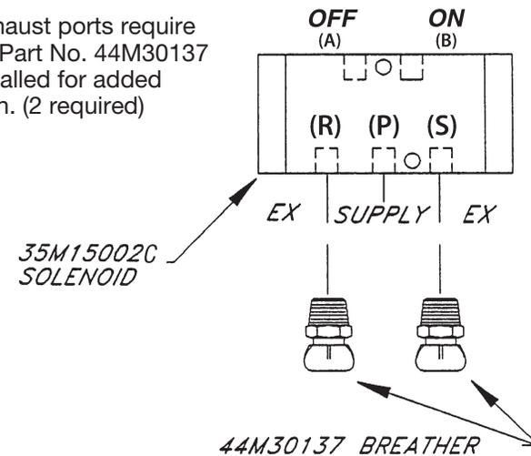
Slightly different fittings may be required to hookup air lines when solenoid is used as a field replacement.
