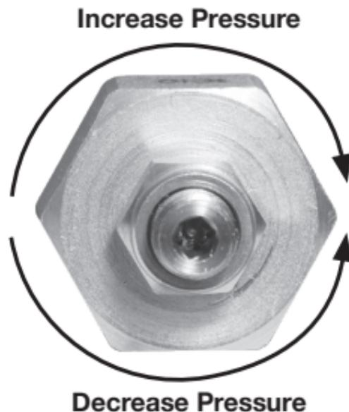
**Pump Relief Valve should be set 100 PSI higher than any secondary relief down stream in system.**
