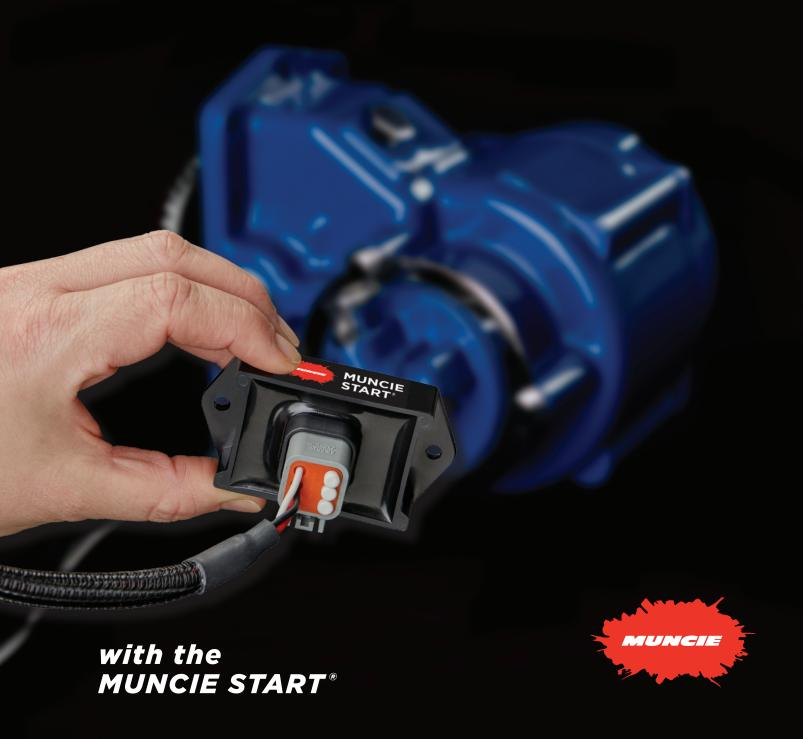
MUNCIE START® is an electronically controlled, modulated clutch engagement system by Muncie Power. It eliminates torque spikes through the power take-off, truck drivetrain, and mounted auxiliary equipment during startup of high-inertia loads. By allowing for smooth engagement of the power take-off, Muncie Start extends the life of both the PTO and driven mechanical components.
