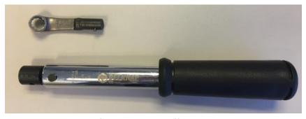
This combination of tools is very effective as it allows improved access to the fasteners, and provides enough leverage to easily torque the fasteners. Since most Muncie PTOs require the mounting fasteners be torqued to 45 lbs ft, this wrench can be used for a wide range of PTO installations.
