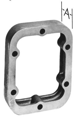
In computing the total thickness of the filler block (spacer) and gasket combination, use a factor of .012" (compressed thickness of a  $\frac{1}{64}$ " gasket 13M35092) for every  $\frac{1}{64}$ " gasket required in installation.
