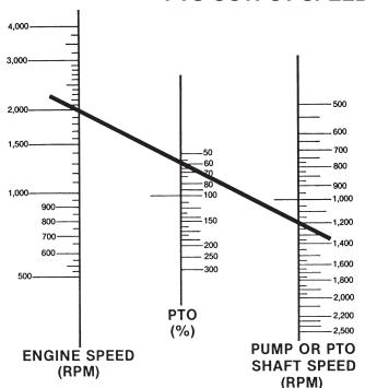
PTO SPEED = ENGINE SPEED  $\times$  PTO%
