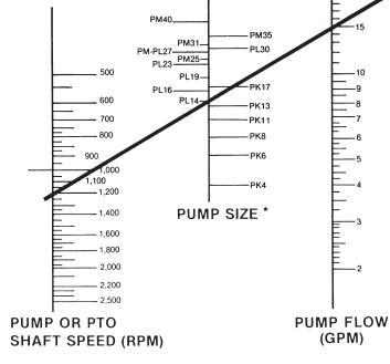
\* Be sure that the pump series you have selected is compatible with the flow and pressure requirements of your system and that it is not operated above or below its rated speed. Refer to page 28 for pump performance ratings.
