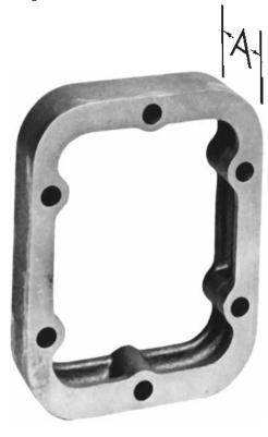
In computing the total thickness of the filler block (spacer) and gasket combination, use a factor of .012" (compressed thickness of a  $\frac{1}{64}$ " gasket 13M35092) for every  $\frac{1}{64}$ " gasket required in installation.
