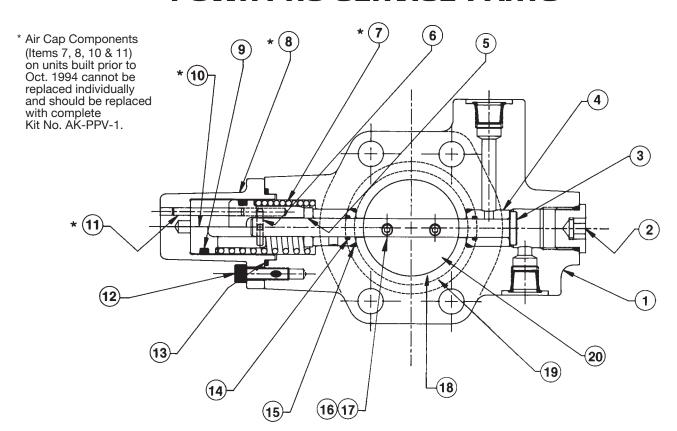
Part numbers shown are for units built AFTER Oct. '94. Older units are not serviceable except for air components.
