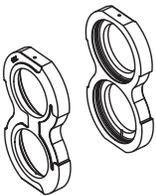
The wear plates seal the gear section at the sides of the gears. Wear here will allow internal slippage, that is, oil will bypass within the pump. A .002" (.05 mm) maximum wear is allowable. Replace wear plates if they are scored, eroded, pitted or discolored. Check the center wear plates where the gears mesh. Erosion here indicates oil contamination. Pitted thrust plates indicate cavitation or oil aeration. Discolored wear plates indicate over-heating, probably insufficient oil.
