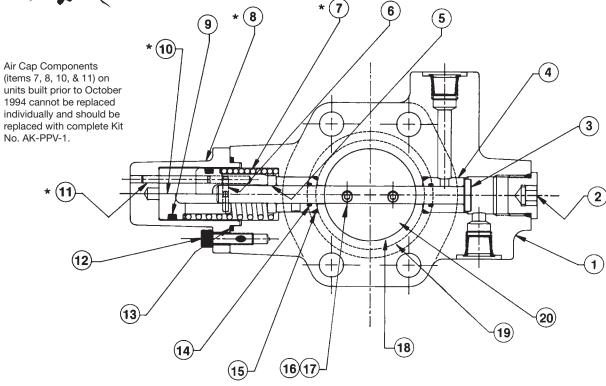
Part Numbers shown are for units built AFTER October 1994. Older units are not serviceable except for Air Components.
