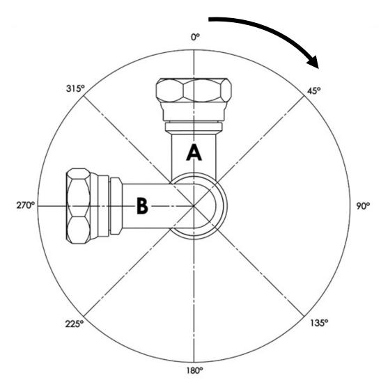
When measuring fitting orientation angle, use the Far End method. Hold the far end fitting (Fitting A) at 0° and orient Fitting B to the desired angle (angles are measured clockwise).
