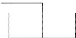
Reservoir, with line below fluid level
