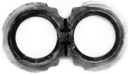
Wear plate showing the effects of overheating
