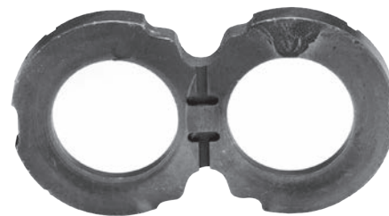
Wear Plate Showing Pitting from Cavitation
