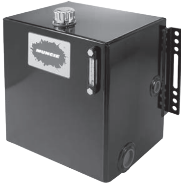
35 Gallon Steel Reservoir (18.25" long × 20" wide × 22" high)
