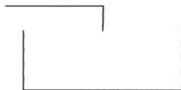
Reservoir, with line above fluid level
