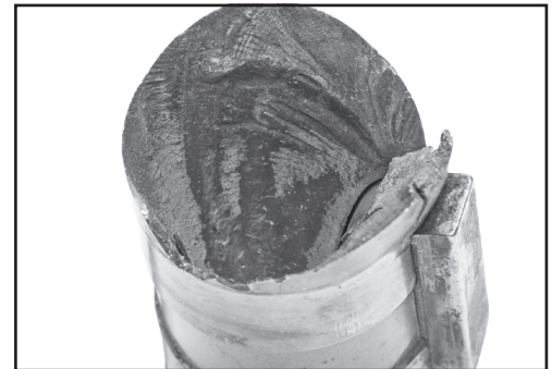
Shaft failure due to cyclic loading
